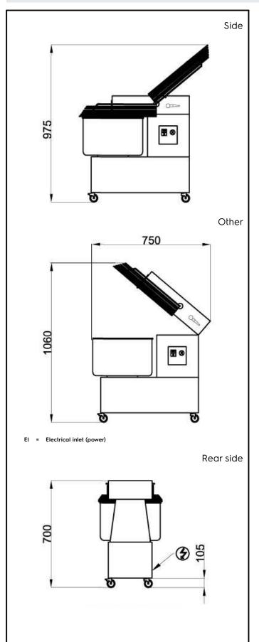
**Electric** Supply voltage: 380-415V/3 ph/50 Hz **Total Watts:** 1.5 kW Capacity: Maximum kneading (60% hydratation): 17 kg/Cycle **Key Information:** External dimensions, Width: 375 mm 650 mm External dimensions, Depth: 700 mm External dimensions, Height: Shipping weight: 89 kg Bowl capacity: 22 lt
